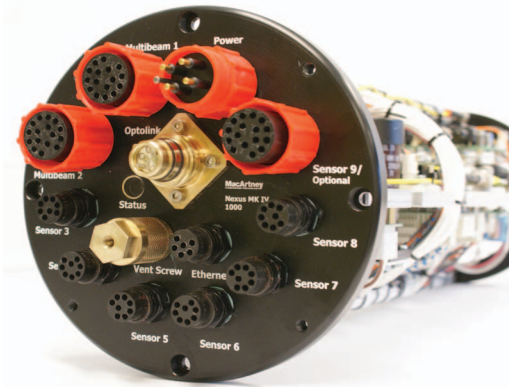
▲ NEXUS MK IV subsea pressure housing bottle ▼ installed on ROV
